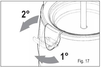
release the bowl from the machine body, using two fingers to prise it away from the fixed steel part of the mixer auger (A) and the others to grip the outer edge of the bowl (B): Gradually pull the bowl harder until it comes away from its seating;
