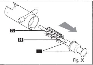
detach the rod (G) from the pin/gasket assembly (I);
