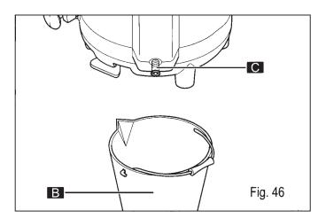
pull out the cap (C) with a firm movement and wait for all the water to empty out from the boiler tank.
