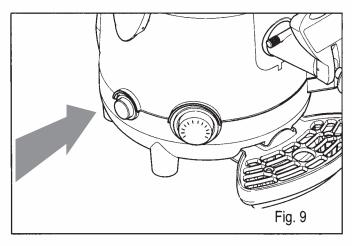
Set the thermostat to the required temperature to heat the product inside the bowl.
