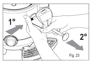
clean the channel connecting the bowl and the tap, using a cleaning brush, as illustrated in the figure;
