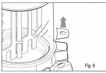
fill the boiler tank with water using the boiler tank level indicator tray, until it reaches the maximum value indicated on the tray itself, which is marked -MAX-:
