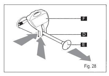
• unscrew the knob (E) by turning it anticlockwise while holding the rod in place;
