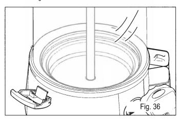
Fig. 37 shows a bpwl which is not correctly assembled; here the bowl does NOT perfectly adhere to the machine edge.
