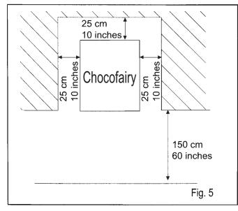
Fig. 5 shows the clearances required for access:
