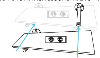
6 ALIGN HOLES WITH WALL ANCHORS AND TIGHTEN FOUR BOLTS, SMALL WASHERS AND LARGE WASHERS IN THE ORDER SHOWN.
