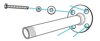
8 SLIDE SHELF ONTO PIPES AND SCREW ON ELBOW NUTS TO FINISH.
