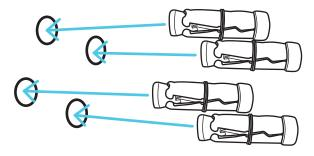
SLIDE SHELF AND REMAINING PIPE ONTO MOUNTED PIPE WITH ROUND BRACKETS ON BOTTOM. USE LEVEL TO ALIGN THE SHELF AND MARK WALL IN BOTTOM THREE HOLES OF LEFT ROUND METAL PLATE. REPEAT STEPS 4-6 TO ATTACH SECOND PIPE TO WALL.
