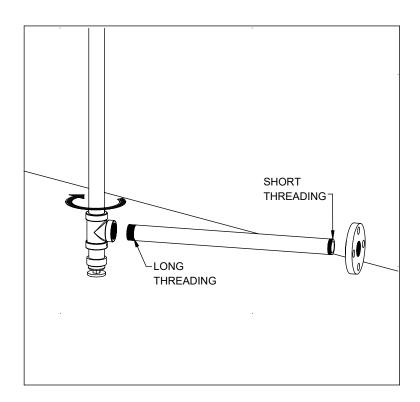
ROTATE THE LOOSE 3-WAY FITTING AWAY FROM THE WALL AND INSTALL A PIPE FLANGE AND SHORT PIPE IN THE SAME WAY AS STEP 1.
