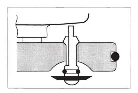
The plastic seals tightly against the cylinder by means of a rubber gasket. The plastic exhaust valve itself can be easily removed for cleaning by light pressure from above.
