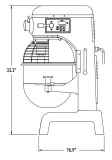
MACHINE ELECTRICAL SPECS: 100-120/50/60/1 – ETL Listed
