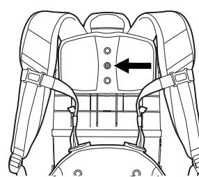
For taller users move the lower adjustment boss upward
