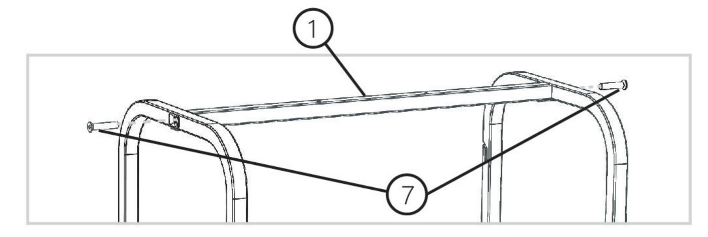
Lay frame on its side and screw in 4 casters, with 4 Lock Washers and 4 Flat Washers. Be sure to install locking casters on front side.
