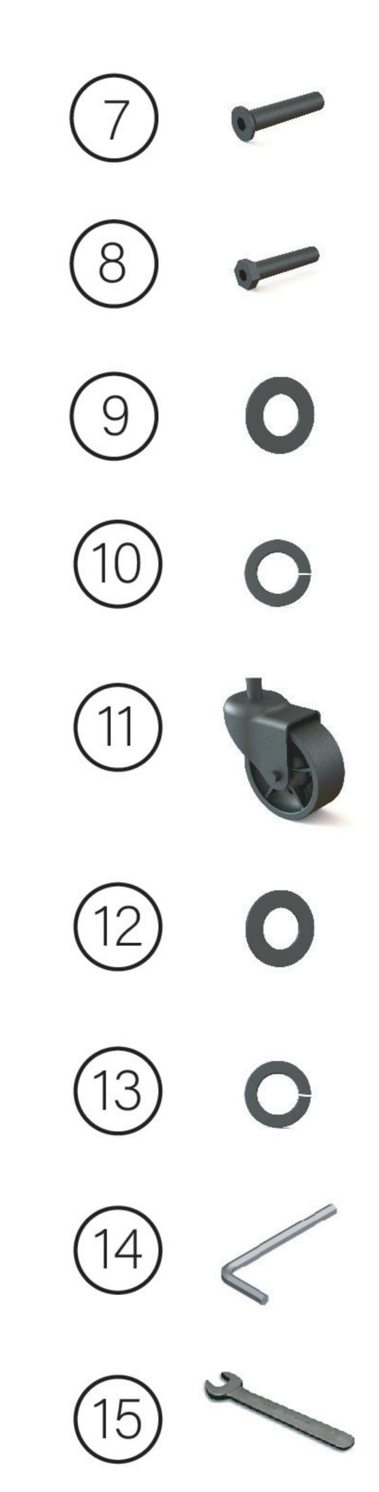
1. Top Bar 2. Tray Shelf x 6 3. Base 4. Sign Holder 5. Left Side 6. Right Side 7. Countersunk Bolt x 2 8. Hex Bolt x 4 9. Black Flat Washer x 4 10. Black Lock Washer x 4 11. Caster x 4 (2 locking) 12. Flat Washer x 4 13. Lock Washer x 4 14. Allen Wrench 15. Wrench
