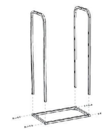
(2) Attach Top Bar to sides as shown with 2 Countersunk Bolts.
