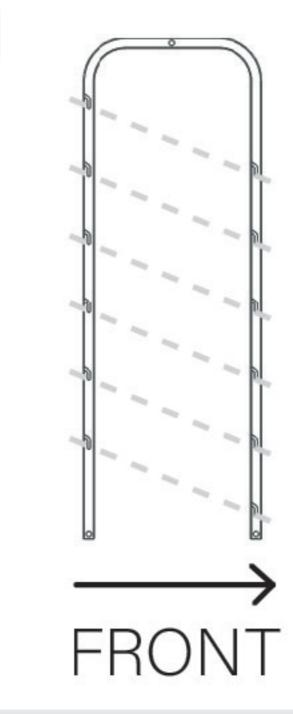
Lift frame upright and install shelves from the back, where the shelf slots are visible, starting with the bottom shelf. Gripping shelf with each hand in the center of one of the horizontal wires, align 4 wire ends with slots as shown and slide forward, then down to secure.
