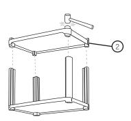
Repeat Step 1 with four remaining Aluminum Pipes(4).
