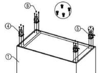
Turn the cart upright. Insert Support Tubing into counter and secure with Bolt A.
