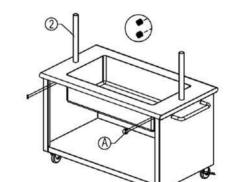
Insert Support Tubing into brackets on underside of Slant Shelf and secure with Bolt A.
