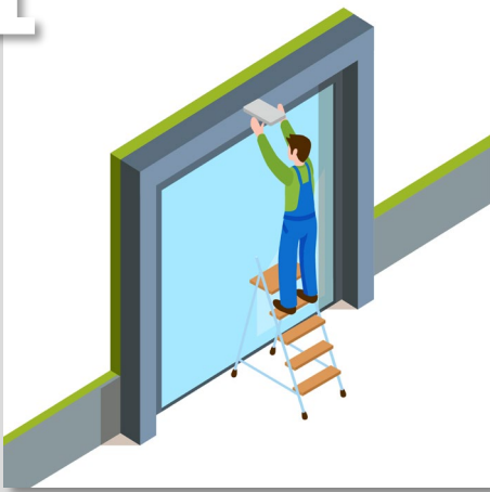
Install SafeCount sensors above entrance and connect cables
