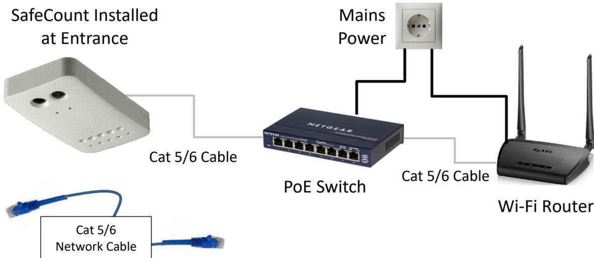
Essentially, the SafeCount device is installed at the door to count people in and out. The IN and OUT values are then used to calculate the occupancy of the building. Note that you'll need a SafeCount device installed at each entrance and exit in order to measure occupancy.
