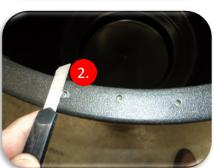
Using a sharp knife, remove protruding plastic from screw holes to ensure a tight seal.
