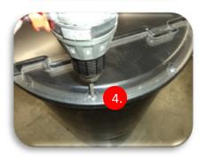
4. Install screws in the 4 provided holes in the back section of the lid.
