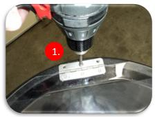
1. Remove the 3 hinge screws using a cordless drill and a Phillips Driver bit or a #2 Phillips screwdriver, remove lid.
