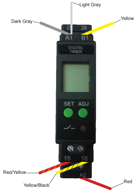
Timer Wiring with Correct Wire Colors
