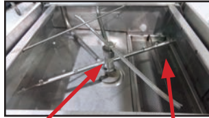
Wash & Rinse Arms, Scrap Screen
