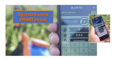
An absolutely remarkable piece of equipment, the Jacto DJB20s "Smart" doser-sprayer utilizes a smart-phone app to create up to 20 various dosage settings between 5 and 300 ml. Doses can be applied automatically or on demand. It's your choice. By using Jacto's "Smart Control" app, doses can be set within 1.0 ml accuracy!
