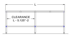
Shipped Standard Welded Set-Up
