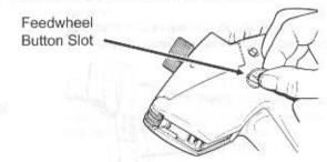
3 Push feedwheel button IN COMPLETELY and turn slightly clockwise if print is too far left or slightly counterclockwise if print is too far right. Adjustment made without completely depressing button are temporary.
