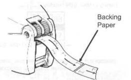
Hold labeler upside down and while squeezing operating lever, feed backing paper into slot. Squeeze operating lever eight times until backing paper comes through the rear exit.
