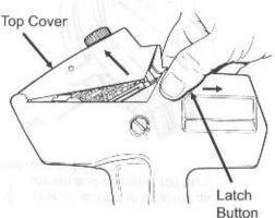
Cut off end of ink roll package. Using package to protect fingers, slide carrier into package and snap new ink roll into carrier.
