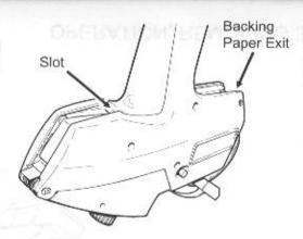
If backing paper does not become taut and exit at rear: Turn labeler upside down, squeeze operating lever and pull backing paper out of slot. Repeat steps, 4, 5, and 6.
