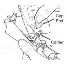
Insert folded backing paper between ink roll and carrier. Pull to snap old ink roll free.
