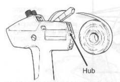
Pull backing paper to the end of the operating lever, separating labels from backing paper.
