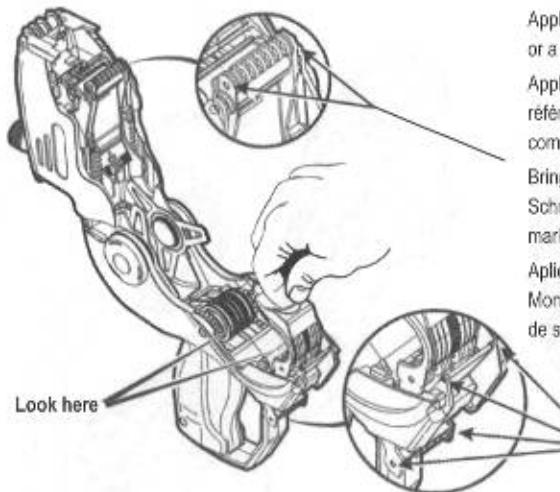
Apply 1 drop Monarch Silicone Lubricant #086989 or a commercial 100% silicone lubricant here.
