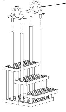
Step 6 **Plant Hanger** Insert Plant hanger tops in 72" legs as shown.
