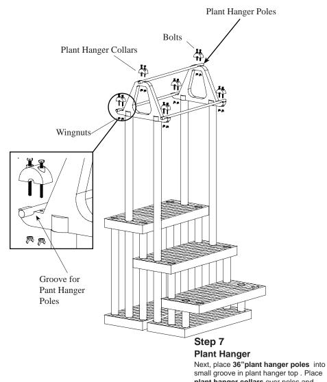
small groove in plant hanger top . Place plant hanger collars over poles and fasten down with bolts and wingnuts.
