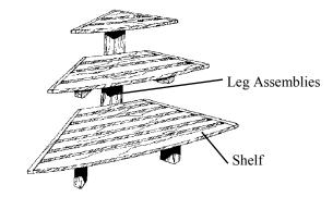
**1.)** Stand leg assemblies on floor and line up at a 90 degree angle so that the two arm extensions on 2" x 2" leg over lap the 2" x 4" leg. Insert two 2 1/2" screws through pre-drilled holes in 2" x 4" leg. Insert 2 - 1 1/2" screws through pre-drilled holes in 2 x 4". Insert 2 - 2 1/2" screws through pre-drilled holes in bottom arm and attach to 2" x 4".
