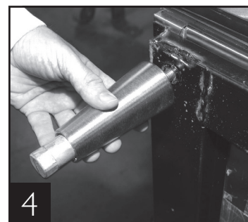
4 Thread leg into cabinet bottom frame rail.
