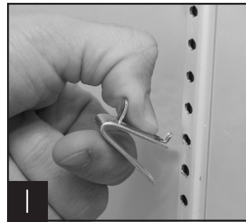
1 Installing top tab of shelf clip
