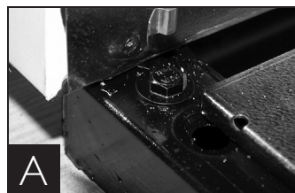
Removing skid from bottom of cabinet.
