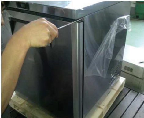
1) Unscrew the top hinge.
