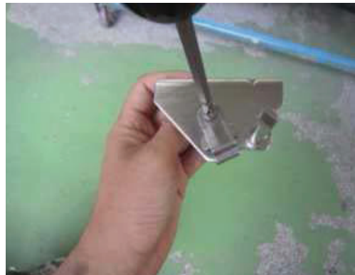
C-2. Disassemble bottom hinge (left).
