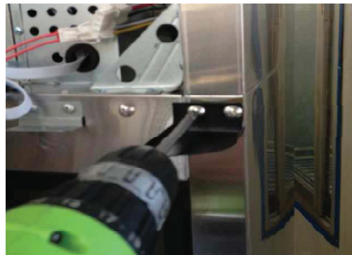
I. Assemble top hinge (right) with fixtures in original positions.
