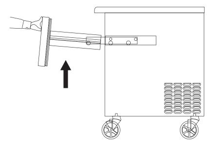
Fully extend the drawer out toward you as pictured. After full extension, lift the drawer up and pull toward you. This will disengage the rollers from the roller guide.
