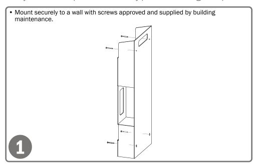
• Dispenser can be mounted to a Bowman Wall or Door Hanger through cutout in back. (See guidelines for door hanger mounting on the hanger instructions.)
