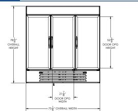
\*NOTE: Remote units are field wired and come with 6" legs. Refrigerant must be specified at time of order.
