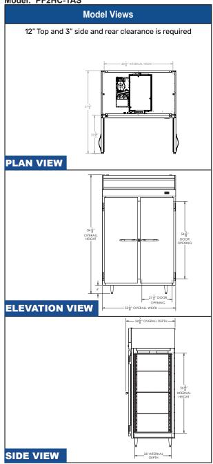
\*NOTE: Remote units are field wired and come with 6" legs. Refrigerant must be specified at time of order.
